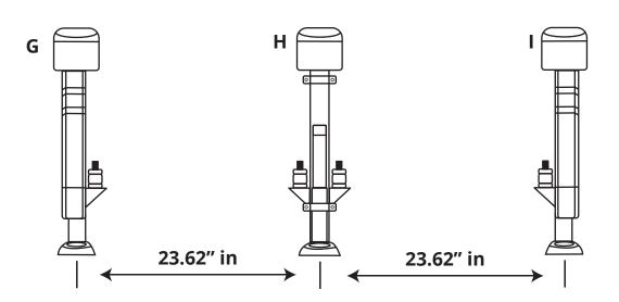
Place **Right Chair Leg (G)** into the desired placement (do not attach to floor). Measure 23.62" in (600mm) then place the **Middle Chair Leg (H)**. Measure 23.62" (600mm), then place **Left Chair Leg (I)**. Measurement is from centerline bolt to the next centerline bolt. Repeat for as many chairs as needed.
